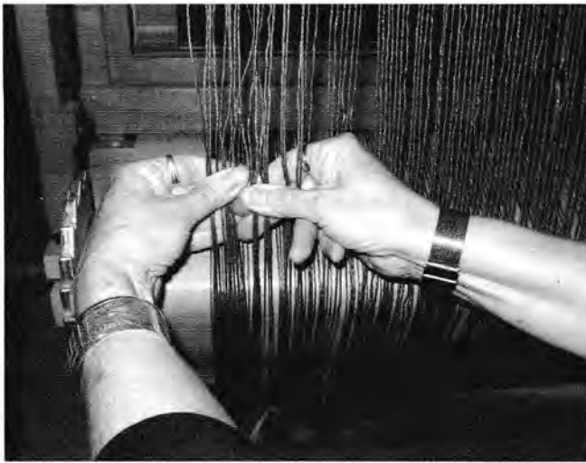
Pull on small sections of warp to fine tune the tension on a long warp.
